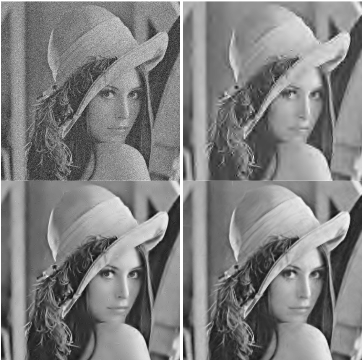
Figure 4: Noisy image (top left) and filtered images using the decimated wavelet transform (top right), the undecimated wavelet transform (bottom left) and the curvelet transform (bottom right).
